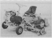
cutting width, and the height of the cut can be adjusted from 1/2 to three inches. The cutting units can be raised or lowered from the tractor
