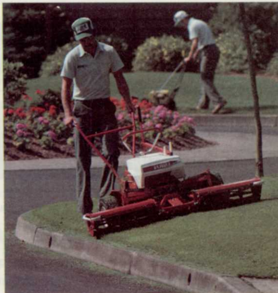
Steve Bizon behind the Toro tee mower he modified to a walk-behind.
