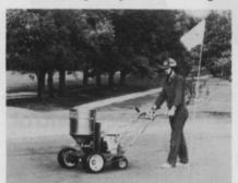
propels the spreader at speeds of up to 2 mph. Finger tip steering controls provide easy steering and excellent maneuverability.
