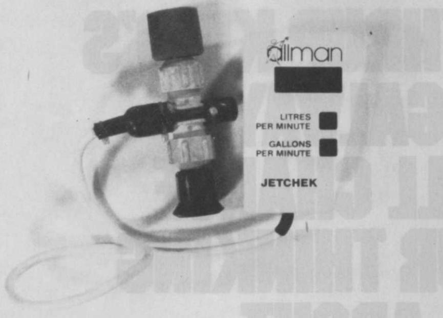
Hand-held device measures flow from a single nozzle instantaneously.
