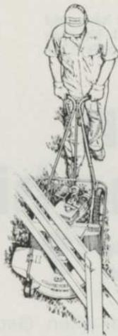
Because the engine is behind the cutting deck, it cuts right down to the water's edge while operator and drive wheel stay high and dry. Cuts grass under fences, branches and shrubs that most mowers can't reach. Belt drive protects from damaging shocks to the engine in case the blade hits obstructions. Dependable 5 H.P. or 8 H.P.
