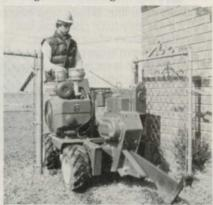
able from Ditch-Witch for burying service lines without trenching. The V252 has four-wheel drive and power steering and features a four-weight vibrator plow with unitrolly assembly. Blade options allow installations with cover from 10 to 13 inches for electric, telephone and television cable and plastic pipe.
