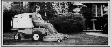
Mows Fast because tractor maneuvers quickly with dual hydrostatic ground drive and lever steering. Many Walker mower owners are reporting their job time is cut 1/3 to 1/2.
