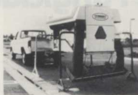
Unit stands alone on legs (included), to free truck for other uses.
