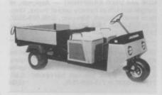
The T2000 is for more rigorous and varied duty. It is powered by an 18 hp twin-cylinder air-cooled Onan gas engine, moving the three-wheel truck through a three-speed transmission at speeds up to 22 mph. Nearly six hours of continuous use are provided by one 8.5 gallon-tank of gas.
