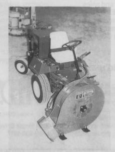
grass clippings, sand and debris off paths, fairways, and parking lots quickly and efficiently. The Model 67 attaches to the Toro Groundsmaster 72 to create a hurricane force wind which can be channeled either direction with a directional chute controlled from the operator's seat. The heart of the Model 67 is a 24-inch diameter fan driven by the Groundmaster's P.T.O.
