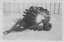
Terra, which can be pulled by an 11-hp tractor, features 140 tines, available in either 1/2-in. or 5/8-in. sizes with a spacing of 3 1/2 to 4 inches.
