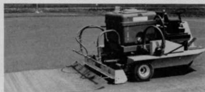
SELF CONTAINED UNIT: Scarifier & Sprayer mounted on the Olathe Turf truck. A complete ATHLETIC FIELD MACHINE!
