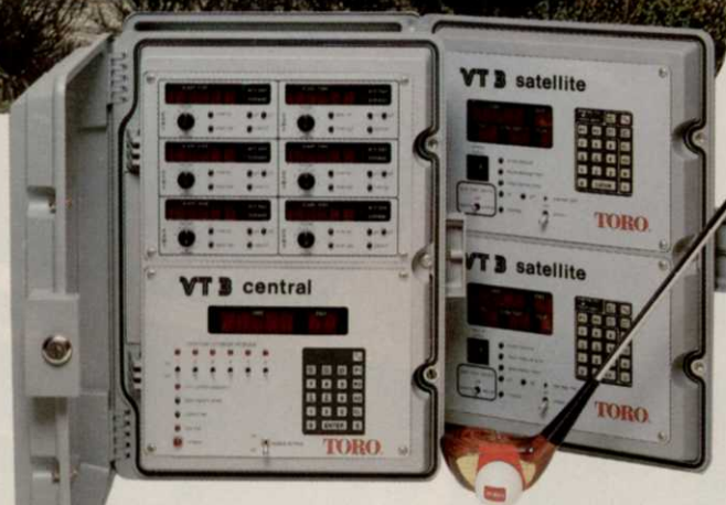
Toro's VT3 central-satellite control system utilizes solid state electronics for accuracy and dependability
