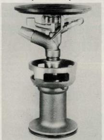
replace the Toro 690 gearbox. An adjustable breakup pin on the drive nozzle reduces dry spots close to the head, while seven nozzle sizes with different volume and coverage patterns are available for special jobs. The 10114 has few moving parts and is made of heavy-duty bronze for long wear.
