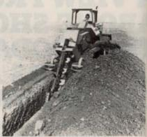
the material to either side of the trench. The conveyor is able to move more spoils than auger spoils delivery systems.
