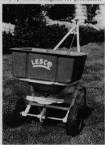
al, multi-use spreading of dry materials such as seed, fertilizer and granular pesticides.
