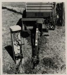
direct burial of power and communications cable and plastic pipe without trenching. For more information, contact Ditch Witch, The Charles Machine Works, Inc., P.O. Box 66, Perry, OK
