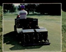
QUICK AERATOR The Quick Aerator's 46" swath covers wide expanses of furf quickly. Choice of 3 time styles: coring, slicing, open
