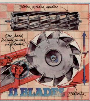
more cutting force. Reduce wheel slippage. Give you smooth, no streak cutting at low heights or in wet grass conditions. We positioned our bedknife optimally near the center line of the
