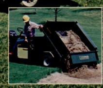
FLATBED BOX & SHORT BOX The Flatbed Box and Short Box attachments haul and dump 1500 pounds of sand or soil, with optional live hydraulics.
