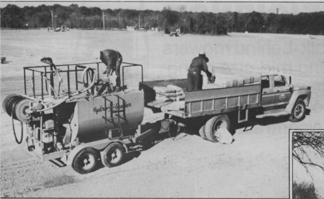
Hydraulic mulching process has saved labor costs because it requires one less worker than blowing straw does. (Below) Freedom Park is one of Charlotte's 91 parks and is one of the oldest.
