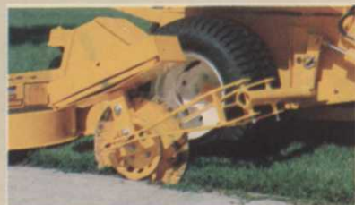
Exclusive coulter-type edger delivers a professional trim.
