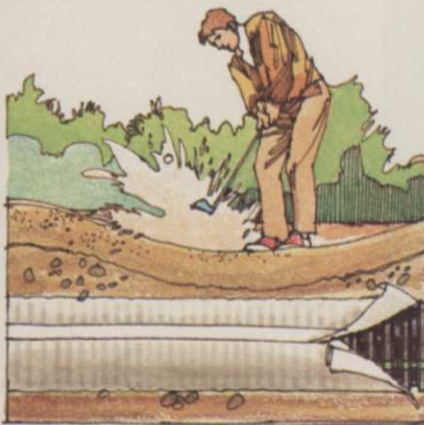
Sandy soils call for ADS Drain Guard®—the nylon filter that won't block or clog.
