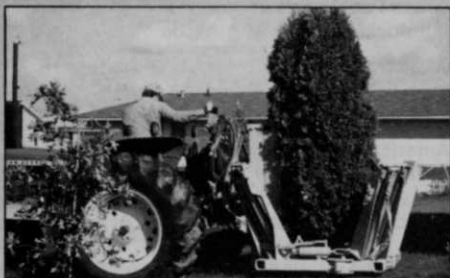
TS-30. Trailer-mounted or tractor-mounted. Ideal for nurseries, tree farms, rental yards and tree service firms. Adjustable towers enable operators to transplant or package either cone shaped or flat-bottom trees or shrubs up to 3" in diameter.
