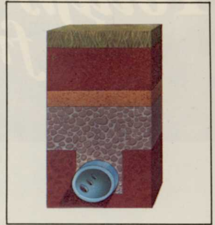
The drainage tile is inset in four-inches of pea gravel, which is then covered with a layer of coarse sand and a foot of topsoil.
