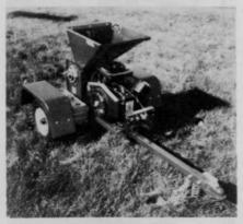
Chipper powered by a 18-hp twin cylinder engine. It offers a rotor design with ½-in. thick cutting knives that can handle limbs of up to 2-in. in diameter. The unit is compact enough to be moved by one man when detached from the towing vehicle.
