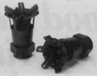
sprinklers made of black sun-resistant nylon with only one moving part. The 5F series offers a maximum coverage of 44-ft. in diameter and droplet size can be controlled, resulting in flow rates from 0.5 gpm to 5.0 gpm.
