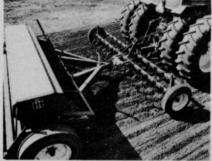
killing small weeds and preparing the seed bed. The cultivator 3-point mounts directly behind rear tractor tires and is about 2-1/2 ft. deep.
