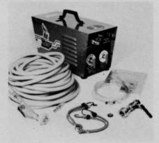
or a tank and injects desired amounts of pesticide or other concentrate directly into the water.
