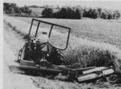
and the mower deck can be locked into a vertical position for road transport. Safety features include shielded universal drive line and belts.
