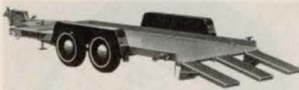
to carry wider and longer loads than comparable 6,000 lb. capacity units. Forged spindle 4-in. drop center axles give a loaded 1406 a low 13-in. ground clearance for increased stability.
