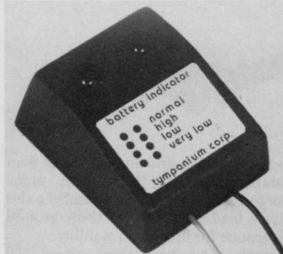
3 malfunctions: amber for insufficient charging, red for overcharging, and both for serious loss of charge.
