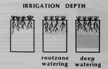
**Fine results** are now being attained by filling the soil to its optimum moisture capacity and to the depth of the root structure of the grasses, and then replacing the daily losses nightly.
