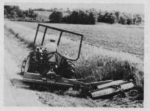
and the mower deck can be locked into a vertical position for road transport. Safety features include shielded universal drive line and belts. Circle No. 165 on Reader Inquiry Card
