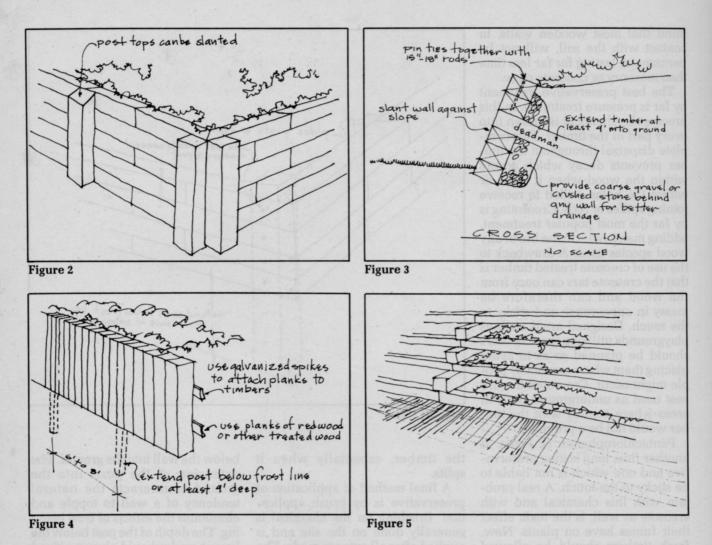
together or for joining the wall to posts. Rods of three-eighth-inch diameter by fifteen inches long can be used also. A galvanized coating will prevent rusting and subsequent failure where moisture is present. Metal straps or angle iron should be avoided as well and can be substituted with strips of redwood or pressure treated woods.
