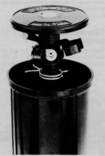
short radius stream and low application rates to resist runoff and puddling. Side and bottom inlets are  $\frac{1}{2}$  in., popup heights is 3 in. and throw range is 14 ft. to 23 ft. A multi-function wiper seal flushes, seals and wipes the pop-up stem.
