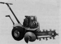
ly replaced hardfaced blades and a screw conveyor to deposit cuttings at the side of the trench. The trencher is compact and easy to operate and has four engine options available.
