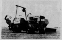
to 60-inches. The four way backfill blade, with replacable grater edge lifts, tilts and angles 30 degrees left and right.
