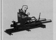
unit may be powered by a Ditch Witch Power Pac 12 or several underground construction vehicles equipped with manifolds.
