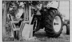
**TS-24.** Compact. Economical. Tractor-mounted. Or, slips onto the forks of most skid steer loaders equipped with an auxiliary hydraulic hookup (with a minimum lifting capacity of 1,200 lbs.). Transplants or packages small trees up to 9".
