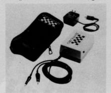
systems. The Checkmate comes complete with test cables, battery recharger and functions for approximately 20 hours on a single charging.
