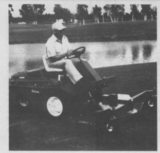
The Performer is available in 18 and 23 hp Power Units, and a selection of 52", 62", and 72" mower decks.
