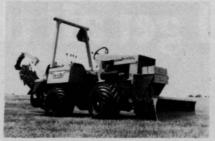
to 60-inches. The four way backfill blade, with replacable grater edge lifts, tilts and angles 30 degrees left and right.
