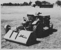
lawn mower at the same time. It comes with standard scoop knives, that cut a width of 46 or 58 inches, and can be pulled by a low horsepower tractor.
