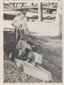
grounds conditions. The single blade is available in 31- or 36-in. cutting widths and the unit is equipped with a 10 horsepower cast iron engine.
