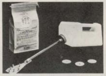
The applicator has a spreader head with three openings that gives a uniform band of granular material 12 to 18 inches wide. The soil sterilant, Urox 5.5, is a free-flowing uniformly granulated product containing 5.5% monuron-TCA which comes in a 10-pound bag. It is best applied just before plant growth begins and should achieve vegetation control for at least eight months.
