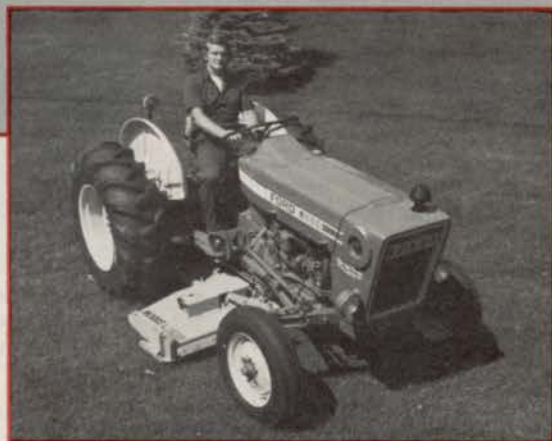
Woods undermounts are adaptable to most tractors rated 15 to 45 hp.
