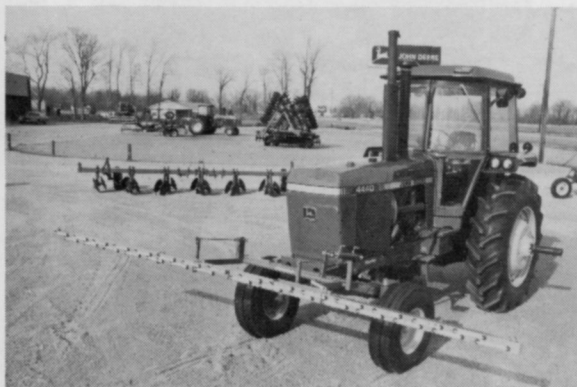
Hustler's aluminum wick bar rubs chemicals directly on weeds, not wasting them on the ground or on turfgrasses.
