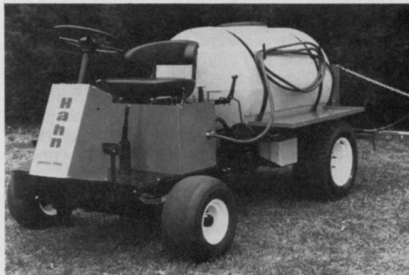
Hahn's Spray-Pro is self-propelled. It has a 160-gallon poly tank, centrifugal pump, and 15-foot boom.
