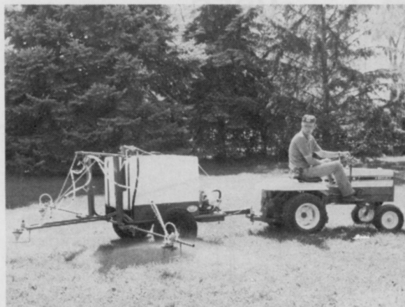
A Broyhill sprayer with MicroMax Rotary Spray Nozzle applies chemicals to a lawn in controlled droplet sizes.
