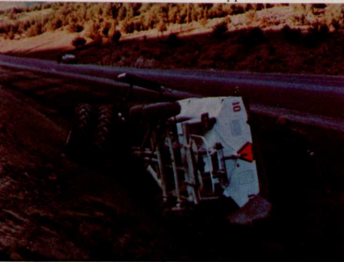
Safety is primary. If the slope is too steep or too rocky, then use other methods of seeding.
