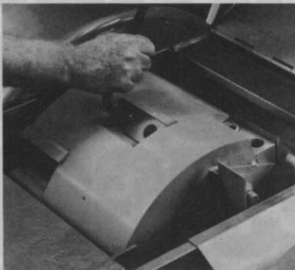
Staggered knife pattern, for years a Mitts & Merrill feature, has always resulted in a lower noise level. First, by segmenting the noise source. Second, through smoother cutting action. Third, by producing smaller chips.
