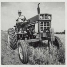
The machine uses a sliding spur-gear transmission with eight speeds forward and two reverse. A category 1, threepoint hitch provides full position control and return to selected depth. A 5.7 gpm pump provides the pressure for all hydraulics.
