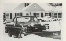
reinforces the blade. Two trip springs on the back allow the blade to "trip" forward and ride over obstacles without damaging the plow or vehicle.
