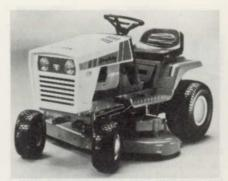
scalping. A quiet-running, twin-cylinder Briggs & Stratton engine and a 42-inch wide three-bladed mower are standard.
