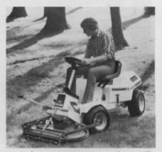
16-inch pneumatic tires, and a totally enclosed engine for a quiet ride. FMC Corp. makes it.
