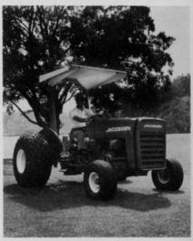
work with its six-speed (plus reverse) transmission. Power range for the G-20's PTO is 30 to 42 hp. at 2250 rpm. Flotation tires roll over moist areas with little turf damage or loss of traction. Operator controls include a tachometer
