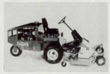
shorter turning radius. A self-adjustment belt-tightening system helps prevent belt slippage in high, tough grass. Optional attachments include 71-inch and 61-inch out-front decks and a cab for the operator's comfort.
