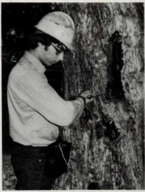
probe's tip contacts decayed wood, readings change dramatically. The Shigometer weighs less than two pounds, making it convenient for checking remote timber stands.
