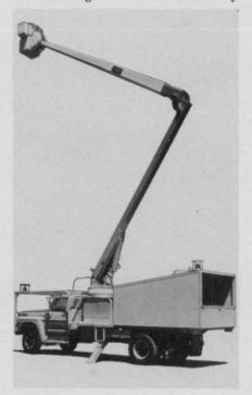
utilities, tree service contractors, and municipalities. Box sizes of 7½, 9, and 12 cubic yards provides versatility. Boxes feature short, flatbed sections that extend under tower pedestals, hinged tailgates, hydraulic dump, lighting and reflective equipment to comply with government codes. Mobile Aerial Towers makes the Hustler II Series to extend 45 feet and the Linesman II Series to extend to 57 feet.
