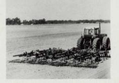
models, the machine includes a flipover hitch with a clevis on one end and a pintle hitch on the other; hand ratchet level adjustment; two spring cushioned front disc gangs set at a 10-degree angle; and 18-inch disc blades with 7½-inch spacing.
