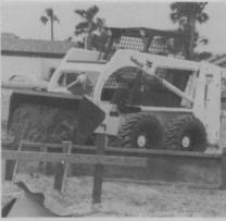
pound operating capacity. At dump height, the models provide 4 inches more reach than the previous series. Different weight distribution results in better loader stability, bucket penetration, and steering control.
