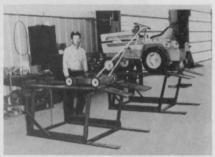
convenient level. Sturdily constructed of heavy gauge pipe and steel, the lift rack carries a maximum weight of 1,400 pounds. Track rails adjust from 24 to 40 inches for different widths of equipment. A safety chain offers protection in addition to the powerful winch that lifts and lowers the machinery.
