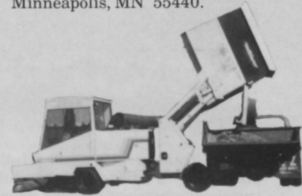
Dumps from ground level to 6 ft.—directly into containers, dump trucks.
