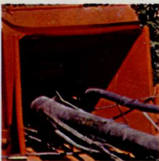
Positive Control feed rolls with instant reverse drive.
