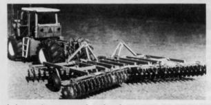
left in the center by the front gangs to insure smooth, well-worked fields. Three hydraulic cylinders control depth and wing folding.
