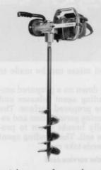
lightweight auger for use by one person. The rugged piece of equipment is available with 4- or 6-inchdiameter augers with carbide flighting and cutting edge.
