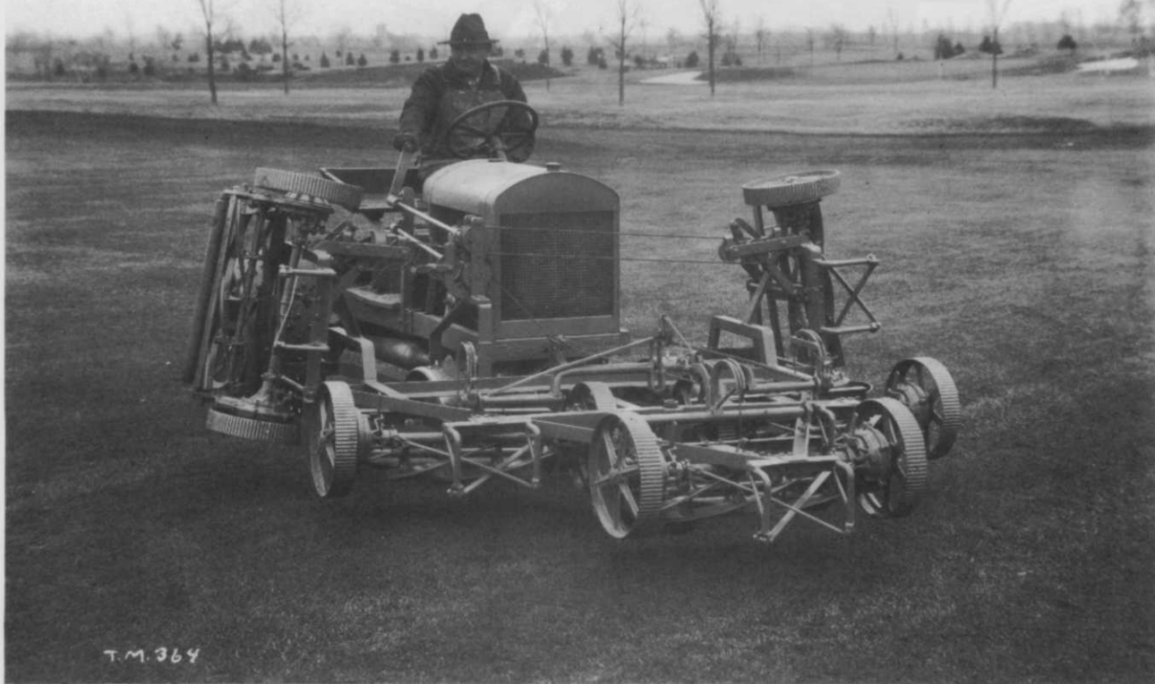
Toro Junior Tractor and five-unit gang mower on well-groomed golf course in 1936.
