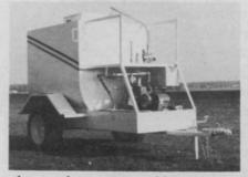
also works as a portable irrigation and pumping system, an auxiliary fire fighting unit, and can resurface ice rinks.
