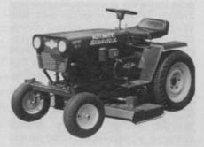
horsepower Briggs and Stratton, cast-iron, electric-start engine, dual range (hi-low) transmission, accelerator-like pedal, foot brake, full hydraulics, and head lights. It accommodates a 48-inch mower deck that hydraulically adjusts to cutting height. The tractor is available with a category 0 3-point hitch.
