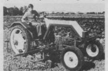
and lowering the tool bar; and a third works optional rear-mounted wheel mark eradicators. A hand throttle in the steering column controls engine speed. A twin-cylinder, air-cooled, 20-horsepower diesel engine powers the vehicle. It has a ground clearance of 19 inches and a track variable from 48 to 76 inches by laterally adjusting the wheels in 4-inch steps.
