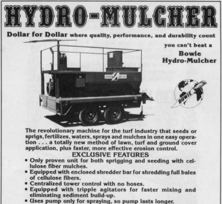
Slurry passes through pump only once, thus reducing seed damage and clogging.
