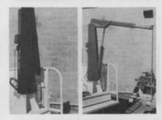
imum vertical reach of over 11 feet. The crane stands 64 inches high above the truck bed in the stowed position. The truck's electrical system powers it and a double acting hydraulic cylinder provides both power up and power down to the boom. GS Industries, Inc. makes the crane.
