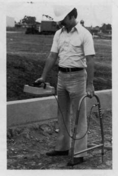
The device locates cables and gauges their depth. Then any damaged section can be found by following the cable and watching the meter.
