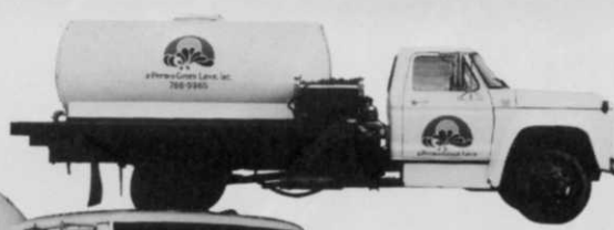
950 gallon fiberglass tank jet spray agitation
