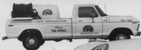
300 gallon fiberglass tank jet spray agitation
