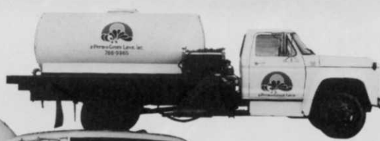
950 gallon fiberglass tank jet spray agitation
