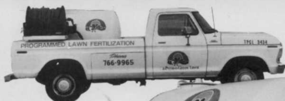
300 gallon fiberglass tank jet spray agitation
