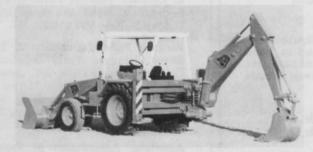
dians, fences, and property lines. It reduces interruption to traffic flow by leaving all lanes open except the one in which the loader is working. Sideshift also gives the operator an unobstructed view of the trench and anyone working in and around the trench. With the backhoe tucked in, there is greater road stability to and from the job.
