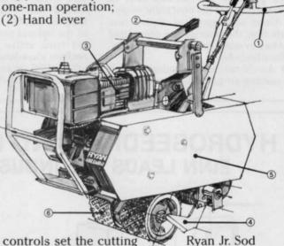
controls set the cutting depth up to  $2\frac{1}{2}$ ; (3) A rugged 7-hp engine delivers plenty of power; (4) You can choose 12" or 18" width models; (5) Its
