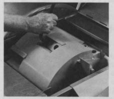
Staggered knife pattern, for years a Mitts & Merrill feature, has always resulted in a lower noise level. First, by segmenting the noise source. Second, through smoother cutting action. Third, by producing smaller chips.
