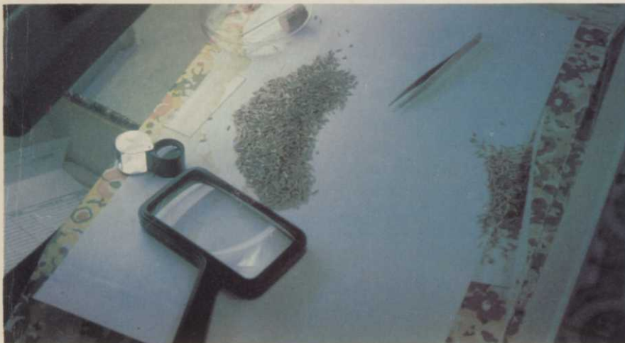
Ten grams of a seed sample are checked for weed and off-type seed in a lab.
