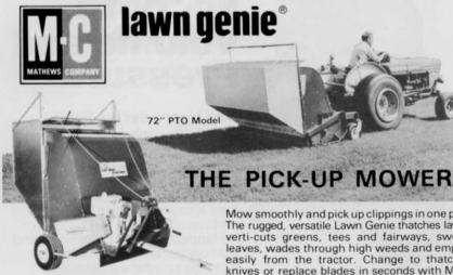
36", 48", 60" and 72" CUTTING WIDTHS-WITH OR WITHOUT LOADING HOPPER Mow smoothly and pick up clippings in one pass! The rugged, versatile Lawn Genie thatches lawns, verti-cuts greens, tees and fairways, sweeps leaves, wades through high weeds and empties easily from the tractor. Change to thatching knives or replace blades in seconds with M-C's patented spring loaded hangers! It's the three season pick-up mower that cleans, mows and sweeps
